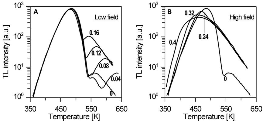
Fig. 4.  $J_{TL}$  curves calculated for various values of the external electric field:  $\Delta E_{\text{field}}$  shown on the diagrams. Transition rate and trap parameters are the same as in Fig. 2. The ‘zero-field curve’ is shown on two diagrams for reference.
