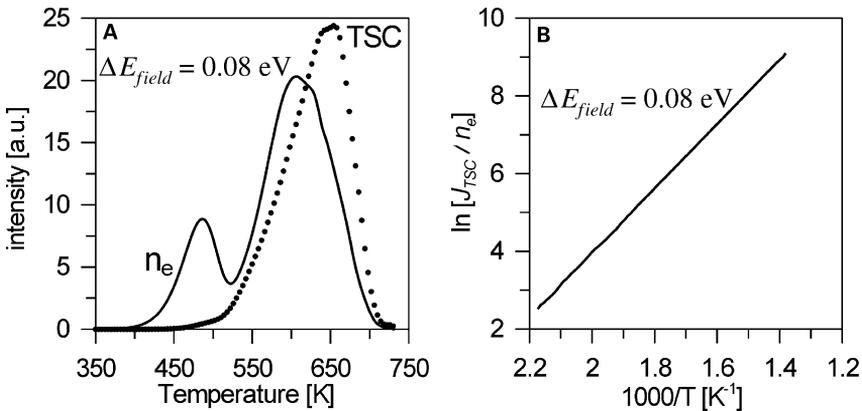
Fig. 3. (A)  $J_{TSC}$ ,  $n_e$  and (B)  $\ln(J_{TSC}/n_e)$  curves calculated for external electric field:  $\Delta E_{field} = 0.08 \text{ eV}$ . Transition rate and trap parameters are the same as in Fig. 2.
