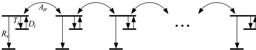
Fig. 1. One-dimensional model for TSC/TL kinetics.  $T_i$ : trapping,  $D_i$ : detrapping,  $R_s$ : recombination,  $A_{tr}$ : transition rate.
